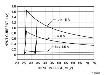
Figure 2. Typical QHW075G1 Input Characteristics at 25 °C
