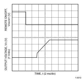
Note: Tested with a 220  $\mu\text{F}$  aluminum and a 1.0  $\mu\text{F}$  ceramic capacitor across the load.
