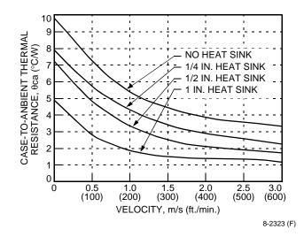
Figure 28. Case-to-Ambient Thermal Resistance Curves; Transverse Orientation
