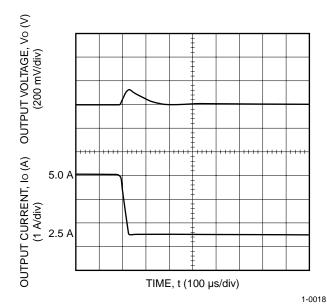
Note: Tested with a 220  $\mu F$  aluminum and a 1.0  $\mu F$  ceramic capacitor across the load.
