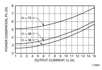
Figure 26. QHW075G1 Power Dissipation vs. Output Current at 25 °C
