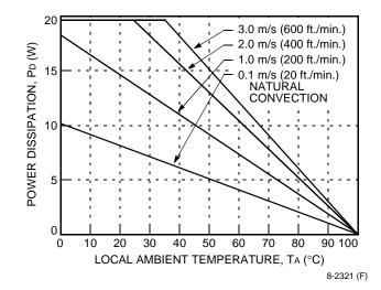
Figure 23. Forced Convection Power Derating with No Heat Sink; Transverse Orientation
