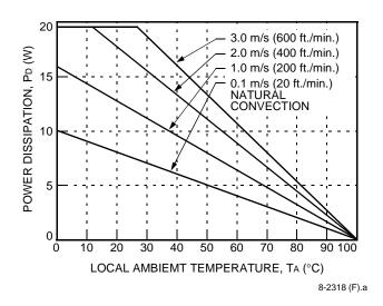
Figure 24. Forced Convection Power Derating with No Heat Sink; Longitudinal Orientation
