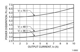
Figure 25. QHW050G1 Power Dissipation vs. Output Current at 25 °C
