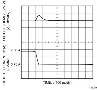
Note: Tested with a 220  $\mu F$  aluminum and a 1.0  $\mu F$  ceramic capacitor across the load.
