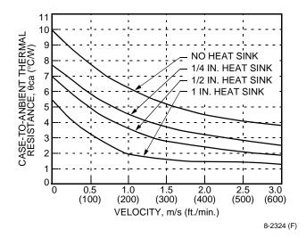
Figure 29. Case-to-Ambient Thermal Resistance Curves; Longitudinal Orientation
