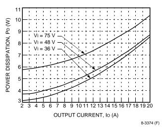
Figure 27. QHW100G1 Power Dissipation vs. Output Current at 25 °C
