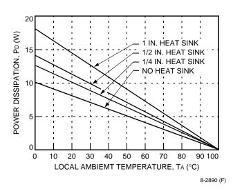
Figure 31. Heat Sink Power Derating Curves; Natural Convection; Longitudinal Orientation
